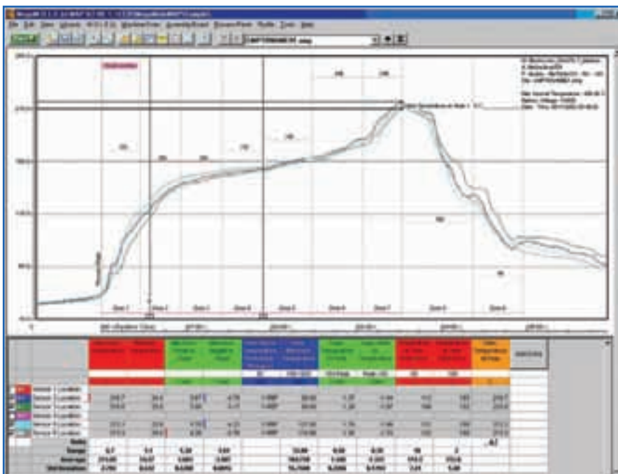
Figure 5. ECD's MAP Software automatically finds and measures the Delta Temp for each profile.
